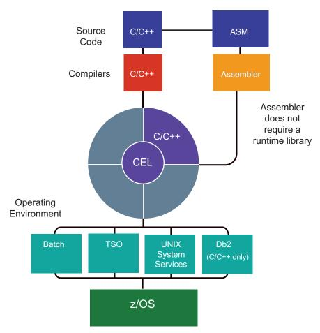
Figure 3. The common runtime environment for AMODE 64
